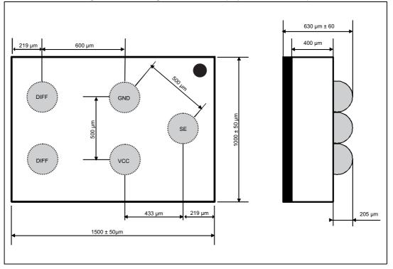
Figure 10. Package dimensions (top and side view)
