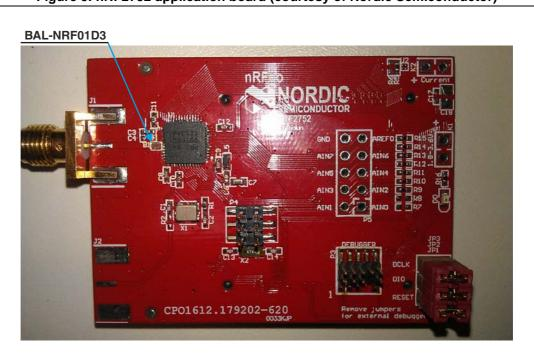
Figure 9. nRF2752 application board (courtesy of Nordic Semiconductor)
