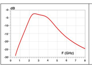
Figure 3. Return loss on SE port (T<sub>amb</sub> = 25 °C)
